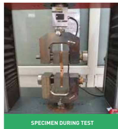
Evaluation of breaking resistance of woodworking joints through tensile shear test according to standard EN 204 (PVA855F based vinyl glue)
