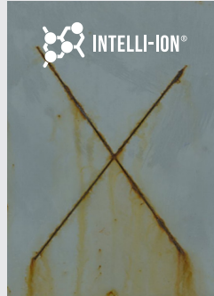
3% Intelli-ion® co-blended with 2% zinc phosphate
