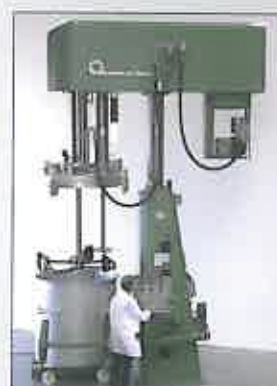
KREIS-DISSOLVER®-BUTTERFLY 90/22 kW, 1500 litres
